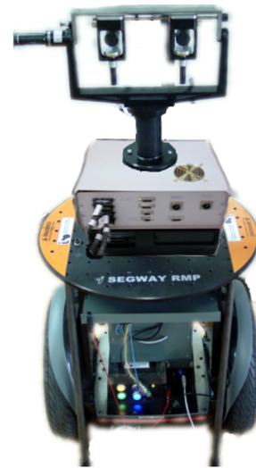
Fig. 1: Four degrees of freedom robotic head mounted on Segway robotic platform body
